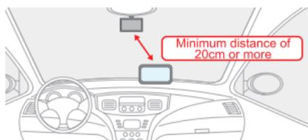
When installing VUGERA with the navigation system, please maintain a 20 cm distance between the two products diagonally. (receiving rate may decrease in some areas with weak DMB and GPS signals)
